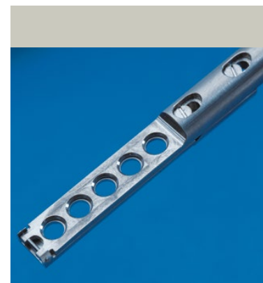
Multiple specimen holder for TEM specimens
