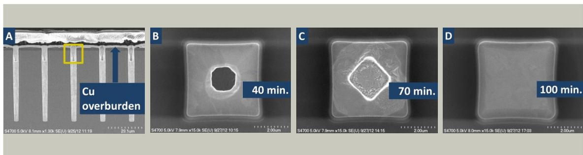
**Figure 2.** FESEM images of Cu TSVs: Cross-sectional view before (A) and plan views (B, C, and D) after removal of overburden.
