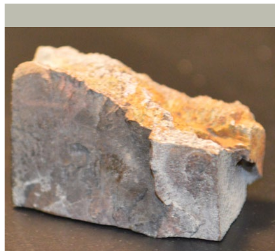
Figure 1. Select a shale sample that is approximately 20 mm \times 20 mm.
